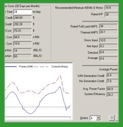
A motor power/current sensor measures both power and current. The test is performed either as a stand alone test or simultaneously with dynamometer data acquisition. The power and current data is processed to determine electrical costs, overall electrical efficiency, gear box torque, power factor, motor loading and other electrical parameters.
