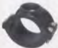
Fig. 90 Service Saddles. WP of 2500 PSIG for pipe 1" thru 4" with outlet pipe size from 1/8" thru 2".
