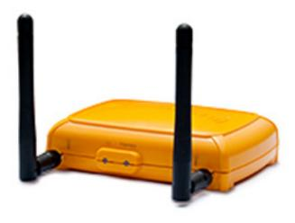
The Wireless Base Station allows simultaneous acquisition of liquid level, dynamometer and pressure records as controlled by the user via the TAM software either at the laptop or at the sensor location.
