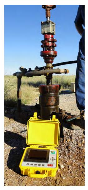
CONVENIENCE FEATURES – The Model H has been designed to facilitate and speed up acquisition of data by minimizing the number of steps to obtain a liquid level depth measurement. This is achieved by setting up the program for the "Quick Shot" mode so that once the instrument is powered up, it takes only three "clicks" to display the signal analysis screen.
