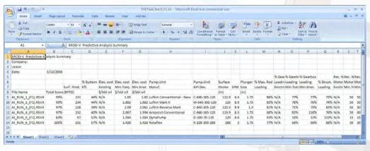
With XROD-V you simply enter the pump depth and a "target" production (or IPR data) and have the program automatically calculate the complete system design (spm, plunger type and size, tubing size, pumping unit size and stroke length, rod string including sinker bars, and motor size). This is done for all the pumping unit types you want to consider. Or, you can select
