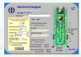
You can either have the program recommend a design for you, or enter your own values for dip tube size and mud anchor size to see what the downward flow velocity will be.
