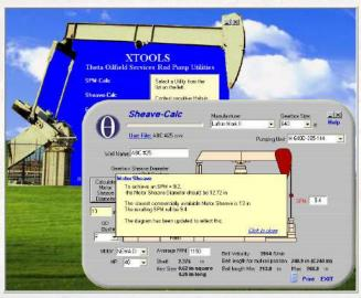
after running RODSTAR to design a new system or to make changes to an existing system, you can use this module to determine what standard motor sheave size you need to get as close as possible to the SPM calculated by RODSTAR.
